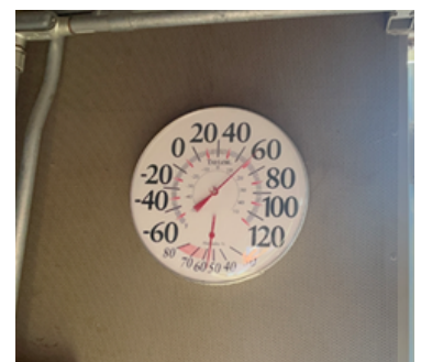
Thermometer mounted inside a temporary enclosure
